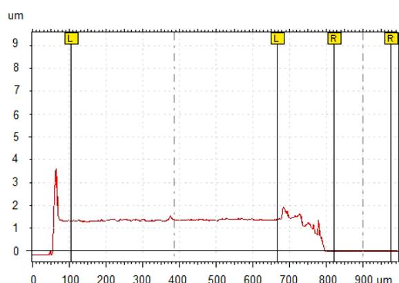
**Fig. 4.** Surface profile of the platinum film coated on glass substrate.
