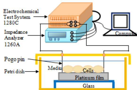
Fig. 2. Experimental setup for cell impedance investigation.
