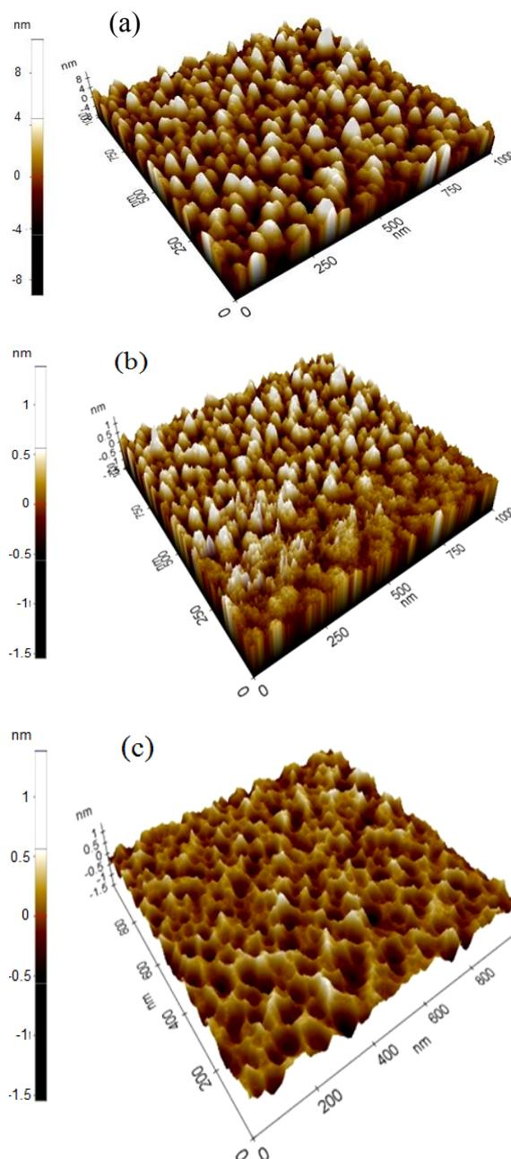
**Fig. 5.** (a) Surface topography with roughness of  $R_a=1.82\ \text{nm}$ , (b) magnetic surface topography at  $R_a=0.223\ \text{nm}$  and the magnetic vortice of (c)  $R_a=0.146\ \text{nm}$ .
