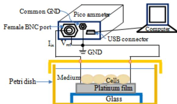
Fig. 3. Experimental setup for cell confluency measurement.
