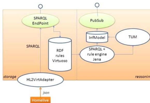
Fig. 4. System architecture.
