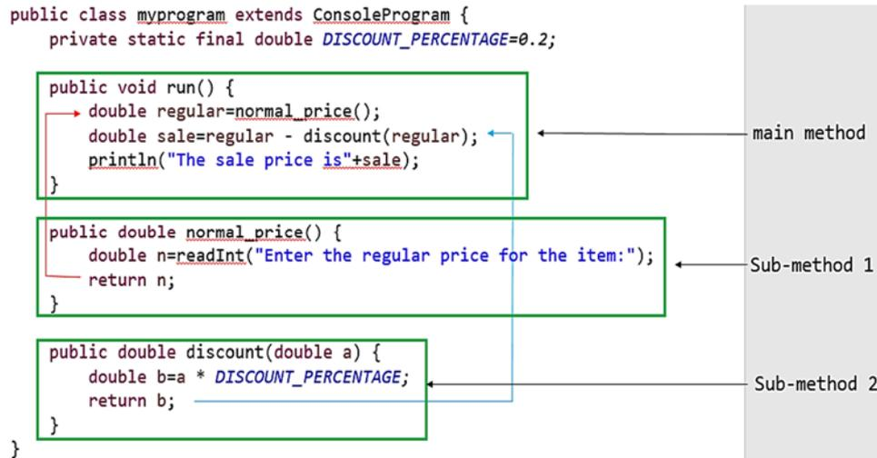
Fig. 2. A Java program example – modularized programming concept.
