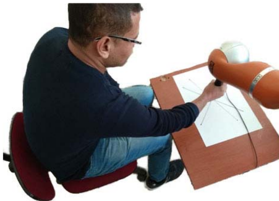
Fig. 5. A simple co-manipulation task in which the best location of both the human-arm and the robot is determined [8, 10].
