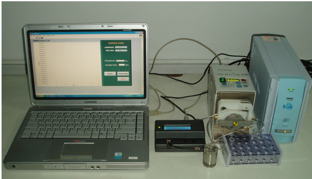
Fig. 2. QCM based DNA biosensor for liquid phase system [6].
