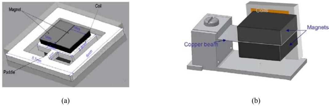
Fig. 9. Generators: (a) Prototypes A/B; (b) prototype C.
