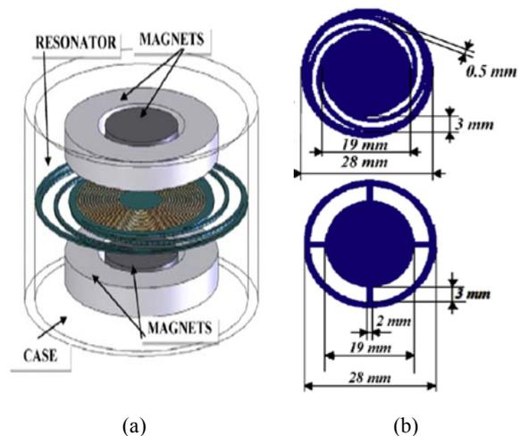
Fig. 3. (a) Generator structure; (b) two resonator structures.
