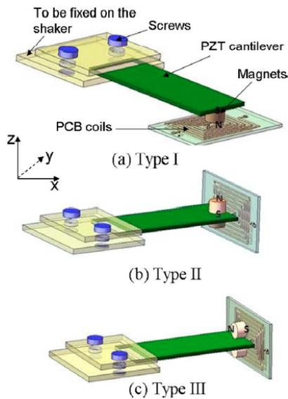
Fig. 11. Hybrid generator (a) type I, (b) type II, (c) type III.
