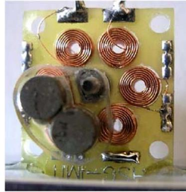
Fig. 10. Generator converts vibration to rotation.
