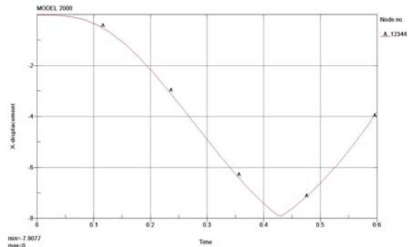
(a) The motion of the sensing mass under the external force 20 g.
