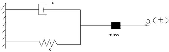
Fig. 2. A simplified model for the low g switch.
