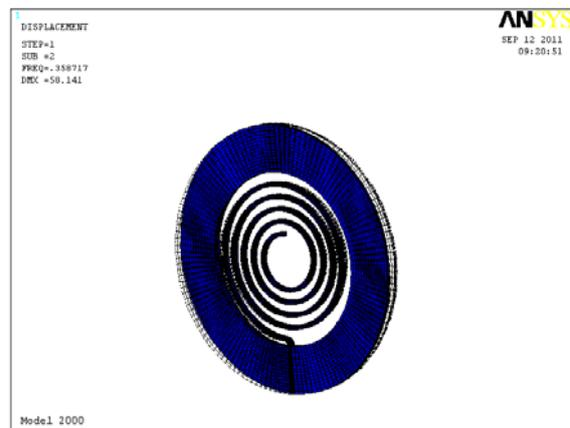
Fig. 6. The 2<sup>nd</sup> order mode shape (f2=358.717 Hz).
