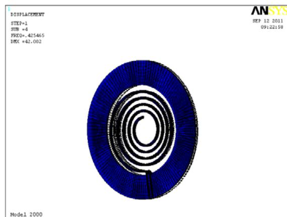
Fig. 8. The 4<sup>th</sup> order mode shape (f4= 425.465 Hz).
