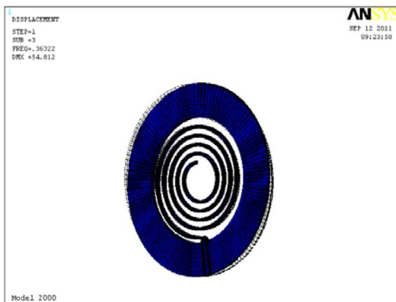
Fig. 7. The 3<sup>rd</sup> order mode shape (f3=363.22 Hz).
