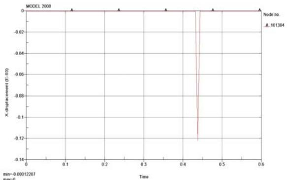
(b) The motion of the fixed electrode during the impact.
