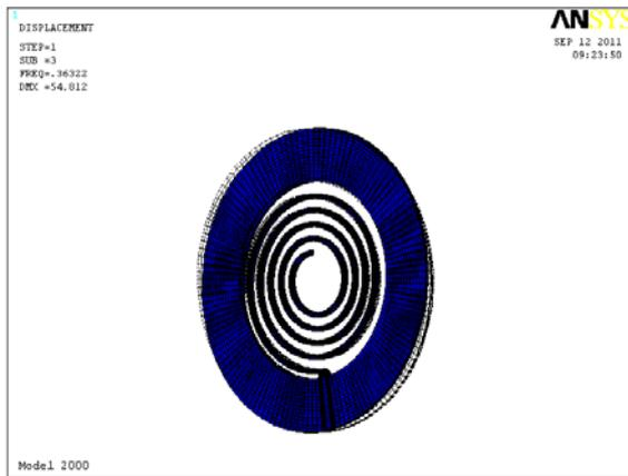
Fig. 5. The 1<sup>st</sup> order mode shape (f1=304.408 Hz).
