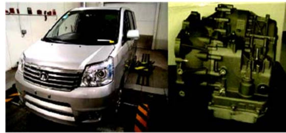
Fig. 7. Test vehicle and Shengrui 8-speed transmission prototype.
