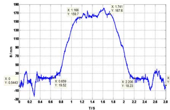
Fig. 9. Test results of axial shifts of the manipulator.
