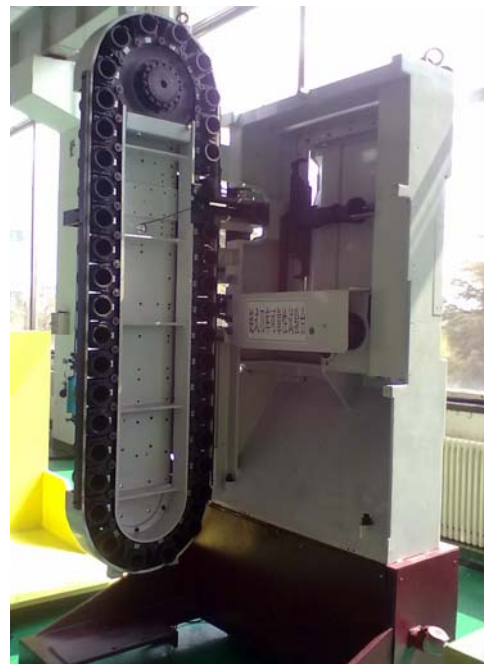
Fig. 1. LS series chain-type magazine.
