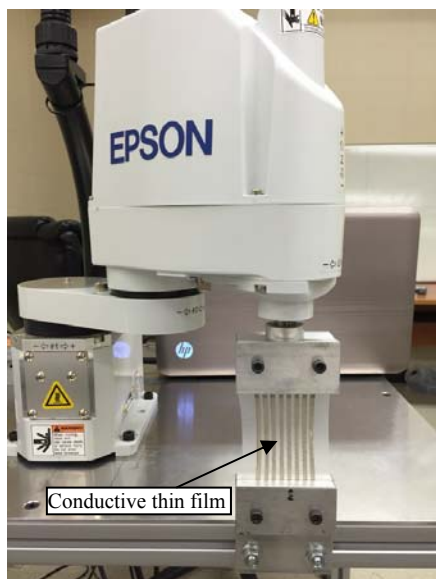
Fig. 3. Fatigue test setup.
