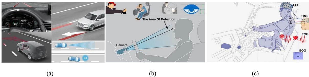
**Fig. 1.** Illustration of (a) vehicle behavioural sensors; (b) driver behavioural sensors; (c) physiological signals sensors for fatigue and drowsiness detection.
