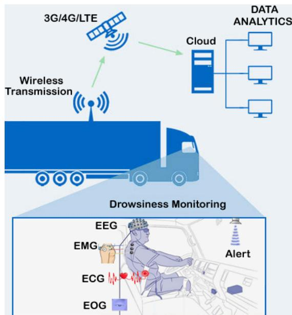
**Fig. 3.** Bio-Sensors Based Driver Drowsiness Detection System Architecture.
