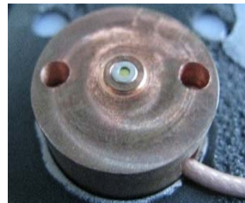
Fig. 7. LD mounted in a copper retainer ring.
