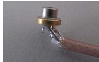
Fig. 6. LD soldered to a formable coax cable.
