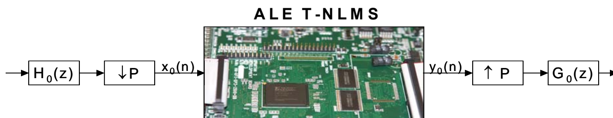
Fig. 7. Block diagram of ALE adaptive filter application circuit.
