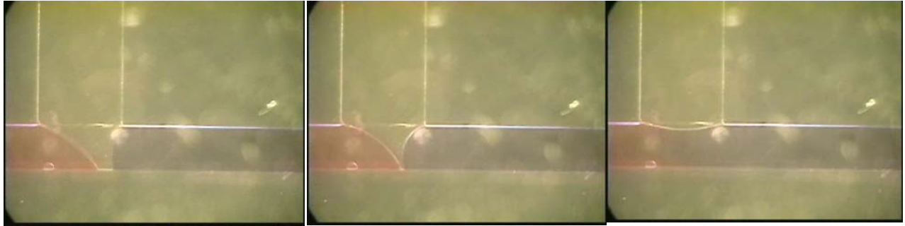
Fig. 1 (b). The trapped air between two drops can be drawn off by a vacuum source connected to the MBV or by applying air pressure from the both ends to push two drops towards the center and the trapped air out to atmosphere via the MBV.
