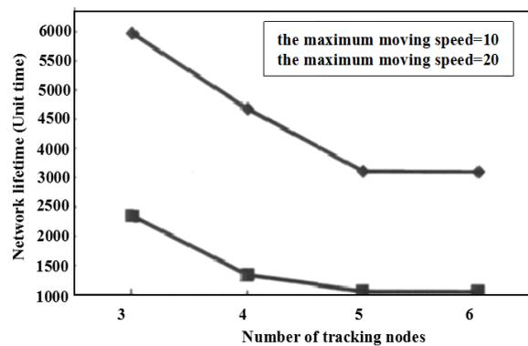
Fig. 5. The target curve motion and linear motion process, the effect of tracking the number of nodes on the network lifetime.
