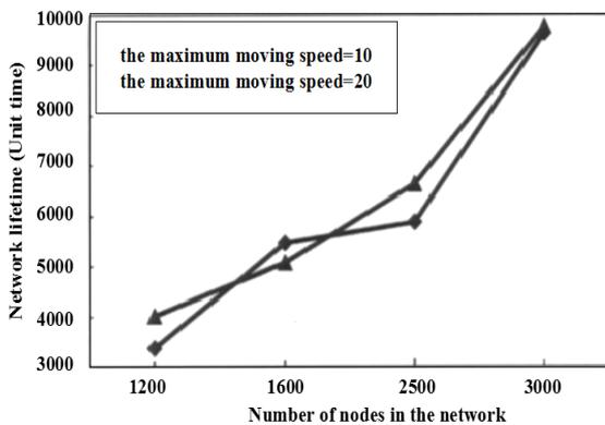
Fig. 1. When tracking number of nodes is 3, the network lifetime suffered the impact of network nodes.
