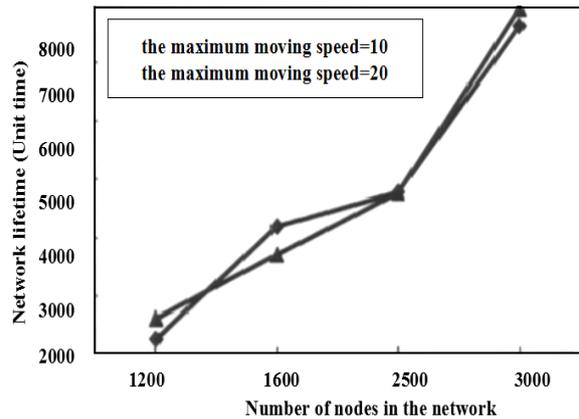
Fig. 2. When tracking number of nodes is 4, the network lifetime suffered the impact of network nodes.
