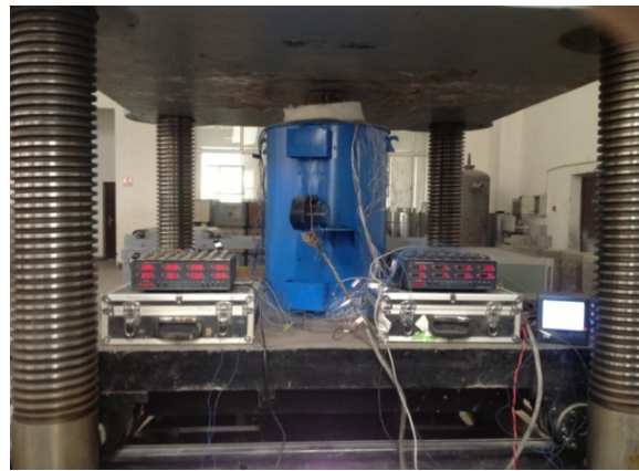
Fig. 6. Test device of thermo-mechanical coupling effect.
