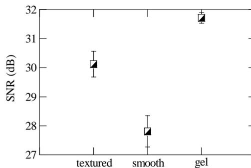
**Fig. 5.** SNR ratio amplitude of textile and gel electrodes.
