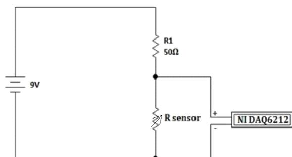
**Fig. 4.** Electrical circuit with piezoresistive sensor and differential connection to data acquisition module.
