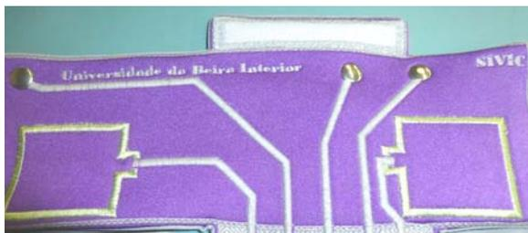
**Fig. 2.** Photo of chest band with interconnection baseplate of neoprene integrating three textile electrodes and two capacitive sensors for the monitoring of EKG and PV signals, respectively.
