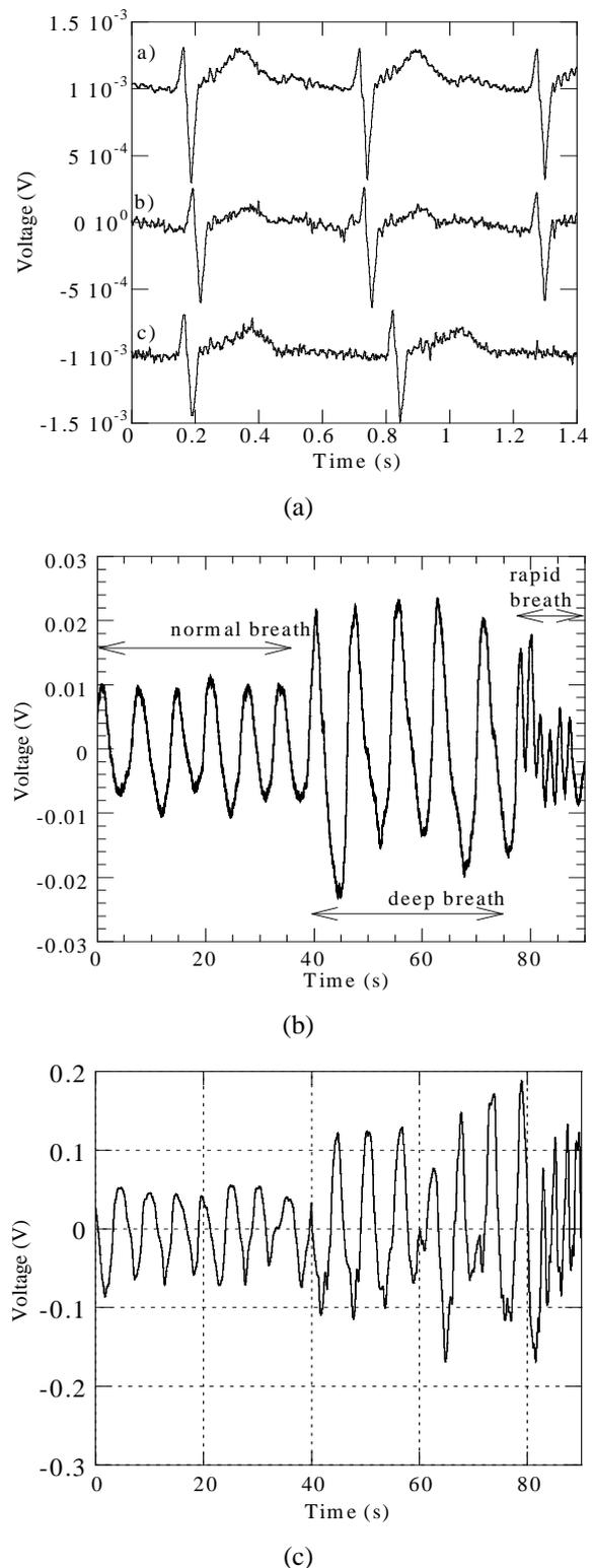
**Fig. 6.** a) EKG waveforms obtained with gel and textiles sensors, where (a) gel electrodes, (b) textured electrodes, (c) smooth electrodes; b) piezoresistive sensor response to normal, deep and rapid breath rates; (c) capacitive sensors response.
