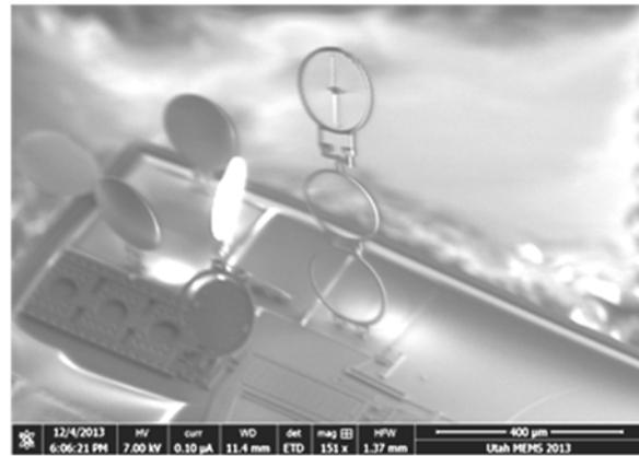
**Fig. 2.** Micro-scale Braun electroscope, fabricated in-plane and deployed by charge pumping from the SEM, showing coulombic effects.
