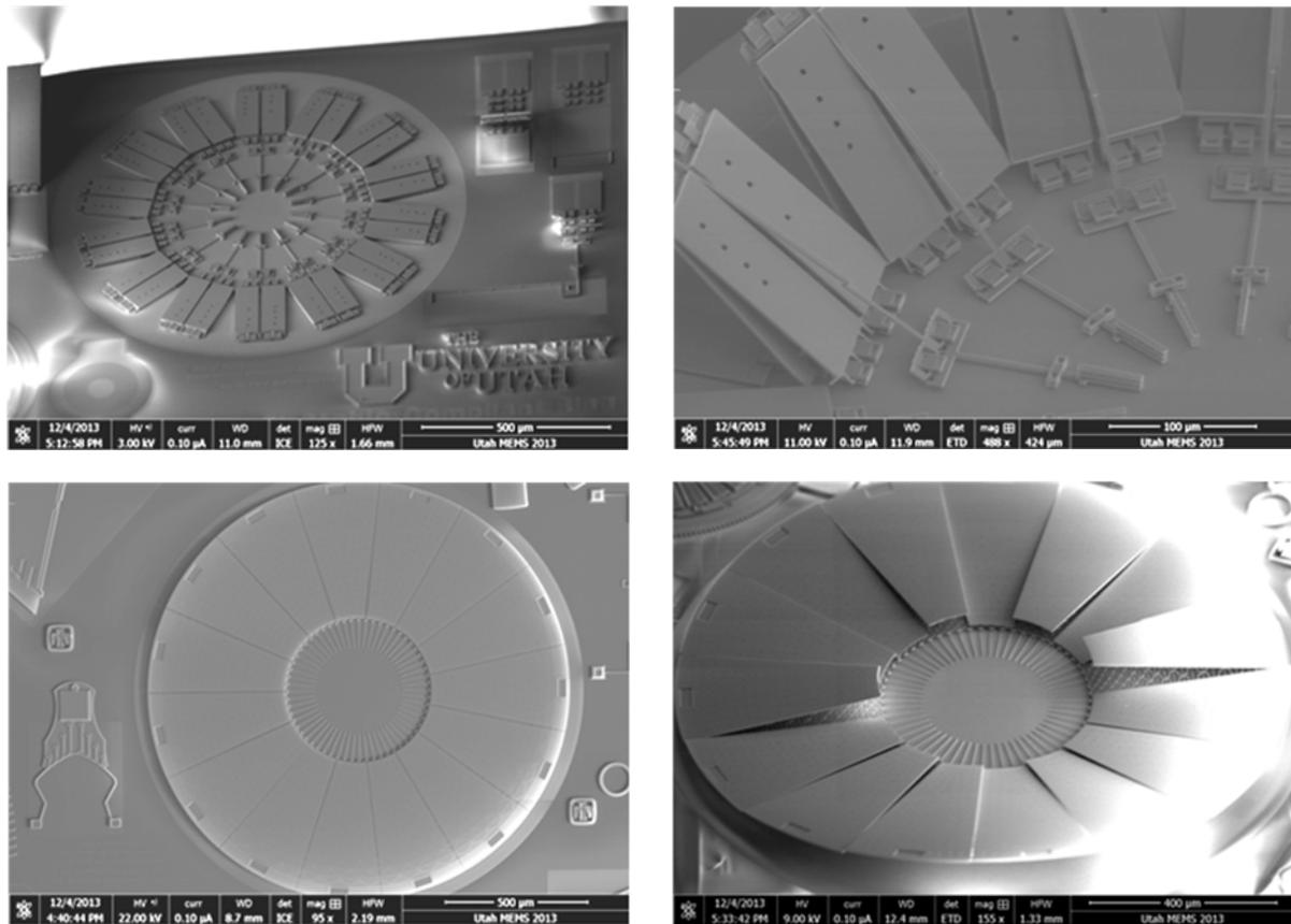
**Fig. 3.** Two versions (upper and lower) of biomimetic lens stretching actuators, (left) base state as-built in-plane; (right) biomimetic lens stretchers actuated out-of-plane by charge pumping. In these cases, the charge pump is the electron beam also used to image the devices. Note the differences in accelerating voltage (HV) between L and R.
