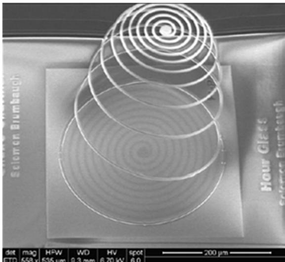
**Fig. 1.** Scanning electron micrograph showing deflection of the spiral beam actuator as observed during SEM imaging. The measured deflection was greater than 1:1 aspect ratio compared to the device footprint ( $220\ \mu\text{m}$  out-of-plane corresponding to an equivalent point load of  $2\ \mu\text{N}$ ) [8].
