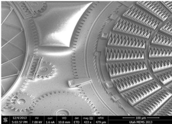
**Fig. 4.** Sandia-designed torsional ratcheting actuator [17] showing voltage contrast in the comb fingers, actuated here by non-contact (SEM) continuous charge pumping.
