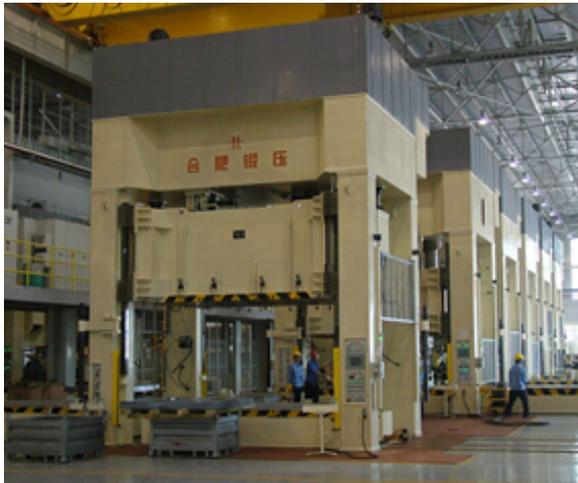
Fig. 1. RZU2000HM sheet drawing hydraulic press.
