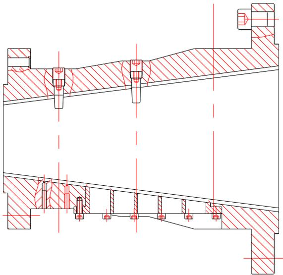
Fig. 2. Dewatering barrel.
