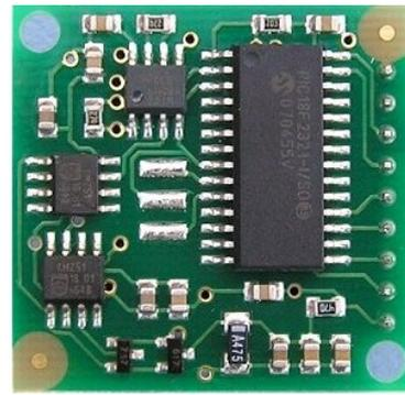
Fig. 9. The compass sensor CMPS03.
