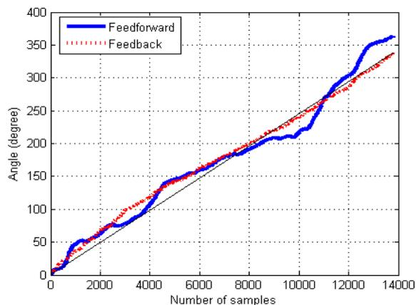
**Fig. 20.** The forward vs. feedback structures in compensating the angle values of the compass when it is placed on a turntable
