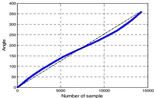
**Fig. 19.** The angle output of the compass sensor vs. the true angle while it was placed on a turntable at room temperature (i.e. 25 °C).
