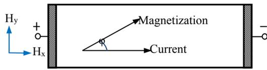
Fig. 3. Formation of  $\phi$  in AMR sensor.
