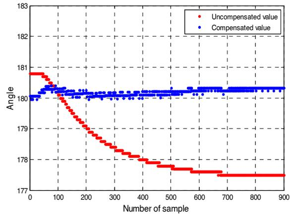
**Fig. 13.** Uncompensated vs. feed-forward compensated values of angles.
