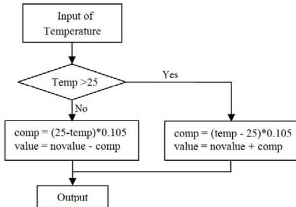
Fig. 7. Algorithm scheme of feed-forward compensation.
