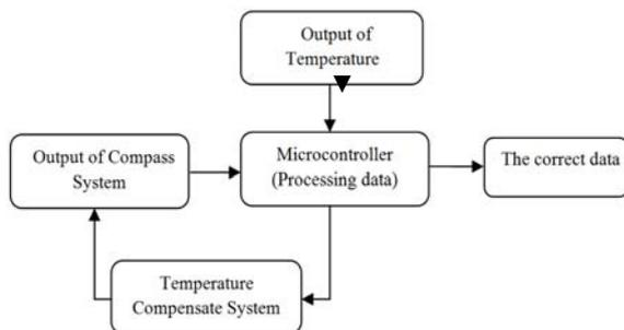
Fig. 8. Block diagram of the closed compensated compass system.
