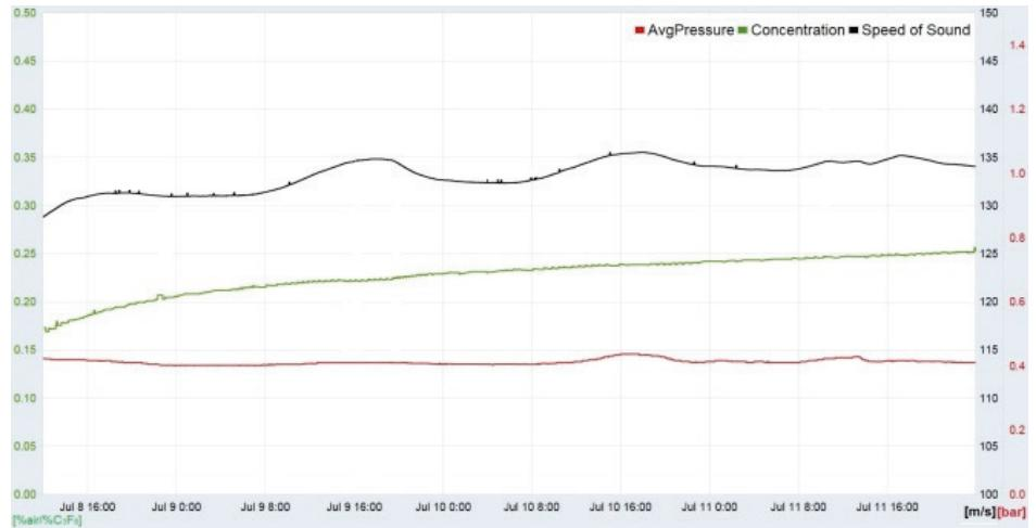
**Fig. 12.** Variation of concentration and speed of sound during the cool-down test (July 08-11, 2016).
