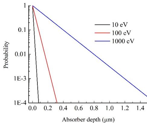
**Fig. 2.** Probability of reaching by a photon a definite depth in the tungsten absorber.
