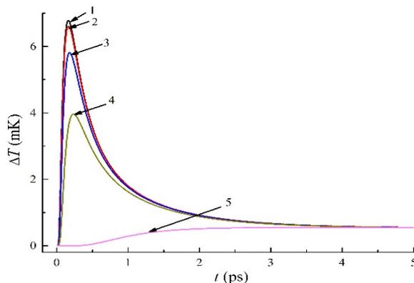
**Fig. 3.** ΔT(t) dependence of the calculation 1M measured in five different areas of the thermoelectric layer: in the center (1), at different distances from the center: 0.2 μm (2), 0.5 μm (3), 1 μm (4), 5 μm (5).
