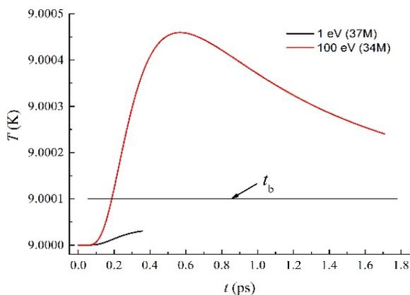
**Fig. 9.**  $T_1(t)$  dependence for 1 eV and 100 eV photons absorptions in the sensors with heat sink of 50 nm thickness.
