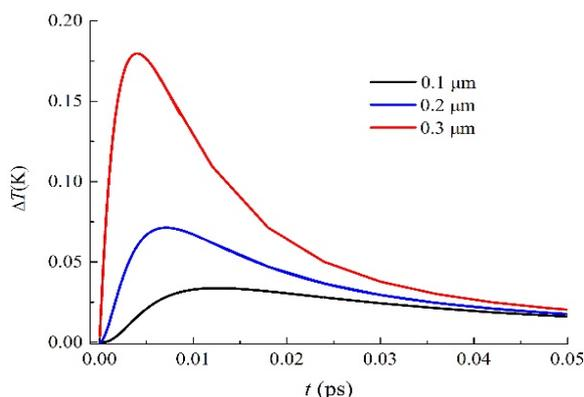
Fig. 7.  $\Delta T(t)$  dependencies of calculation numbers 4 M, 27 M, 28 M for the cases of absorption of photons with 100 eV energy at 0.1  $\mu\text{m}$ , 0.2  $\mu\text{m}$  and 0.3  $\mu\text{m}$  distances from absorber surface.
