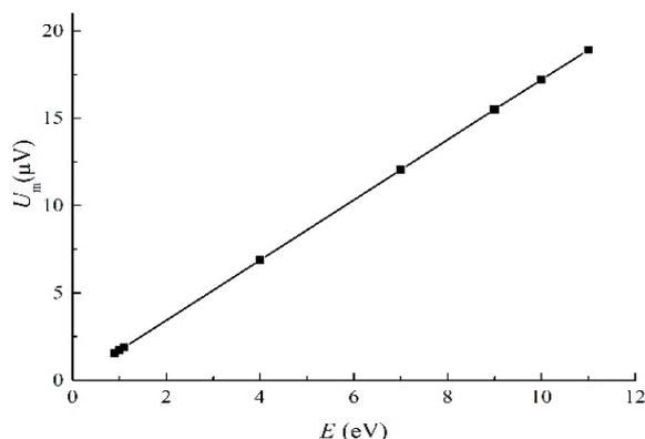
Fig. 6. Dependence of the  $U_m$  parameter from calculations 19M – 26M on the energy of absorbed photon.
