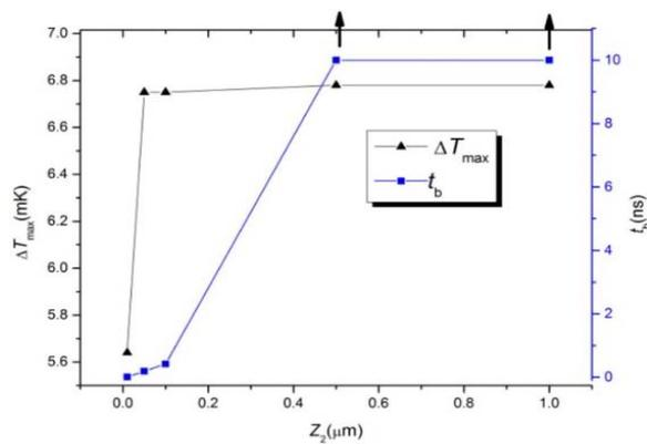
**Fig. 4.** Dependence of the  $\Delta T_m$  and  $t_b$  parameters of calculations 1 M – 5 M on the thickness of the thermoelectric layer.
