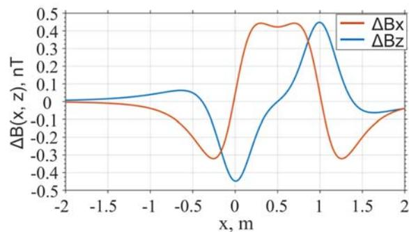
**Fig. 2.** Modeling results for a steel sphere with  $R=1$  cm and  $M_y=M_z=0$ ,  $M_x \neq 0$  with centre coordinates  $x_s=y_s=z_s=0$ , flight at height  $z=0.5$  m along x-direction and  $B_0$ ,  $m=50,000$  nT.
