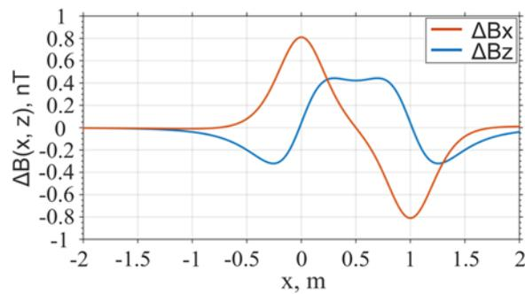
**Fig. 1.** Modeling results for a steel sphere with  $R=1$  cm and  $M_x=M_y=0$ ,  $M_z \neq 0$  with centre coordinates  $x_s=y_s=z_s=0$ , flight at height  $z=0.5$  m along x-direction and  $B_0$ ,  $m=50,000$  nT.
