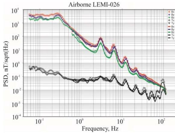
**Fig. 5.** Spectral analysis of LEMI-026 magnetometer noise level when mounted onboard drone at flight.
