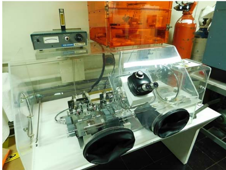
Fig. 10. Sealed chamber under Argon atmosphere, to which the package plastic lid was bonded.
