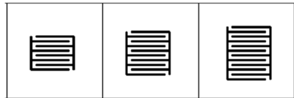
Fig. 3. Configurations of IDC structures with finger pairs of four to six.
