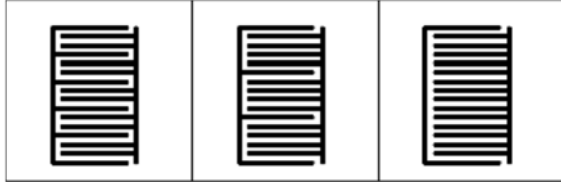
Fig. 6. Configurations of IDC structures with 16 fingers [1_2_1, 1_4_1 & 1_14_1].
