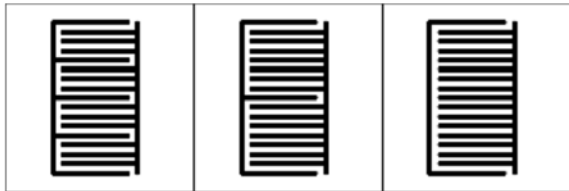
Fig. 7. Configurations of IDC structures with 17 fingers [1_3_1, 1_7_1 & 1_15_1].
