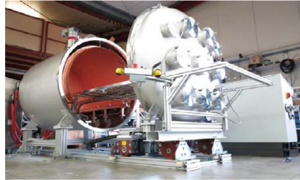
Fig. 5. Photograph of the thermal vacuum chamber for functional and performance tests verification of the phasemeter instrument.
