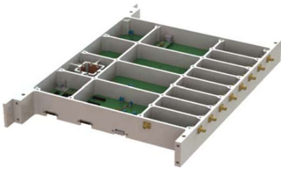
Fig. 3. Illustration of a prototype for the Back-End Electronics Module currently under manufacturing.
