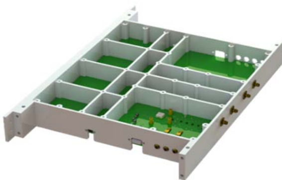
Fig. 4. Illustration of a prototype for the Frequency Distribution Module currently under manufacturing.
