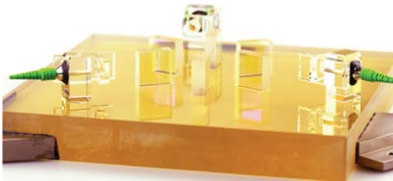
Fig. 7. Photograph of the optical ground support equipment for testing key performance aspects of the phasemeter instrument.
