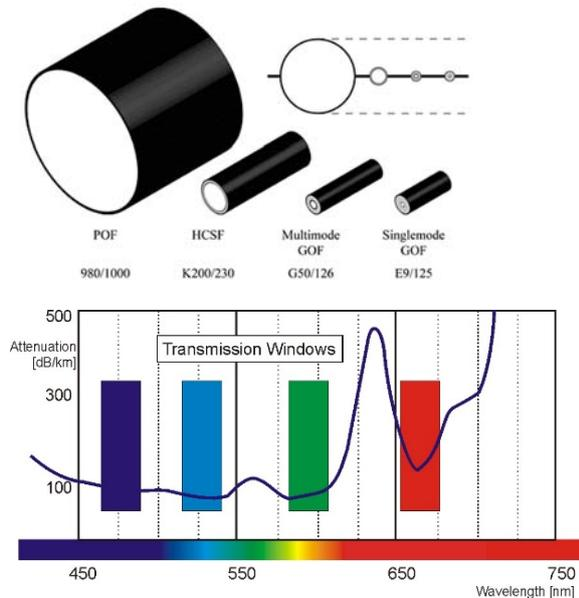
Fig. 1. Principle and attenuation of POF in the visible range [1].
