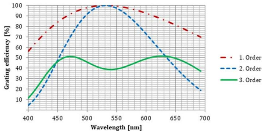
Fig. 4. Grating efficiency for different diffraction orders.
