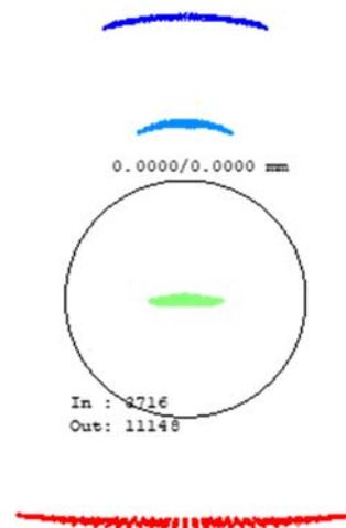
Fig. 6. Spot diagram (optimized, circle diameter 1 mm).
