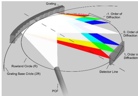
Fig. 2. Principle sketch of a Rowland spectrometer.
