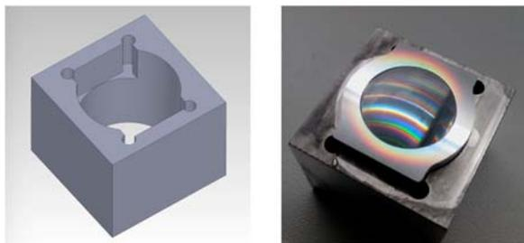
**Fig. 11.** a) Holder for the sputtering process;
