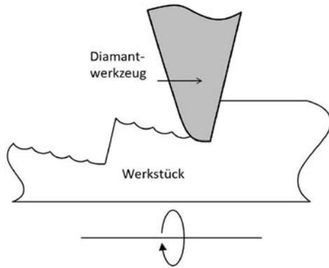
**Fig. 10.** Principle of the grid lines production by marking off the sawtooth structures (adapted from [18]).
