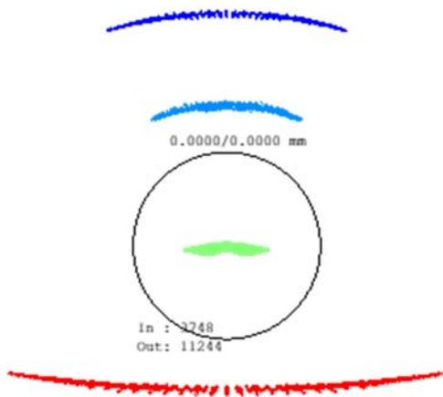
Fig. 5. Spot diagram (not optimized, circle diameter 1 mm).
