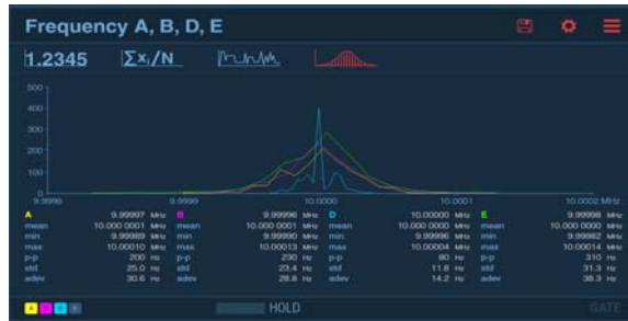
Fig. 5. Simultaneous display of four 10 MHz input frequencies (frequency distribution diagram).
