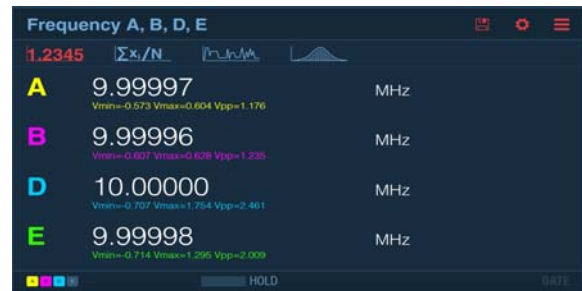
Fig. 2. Simultaneous display of four 10 MHz input signals (Numeric frequency values plus voltage levels).
