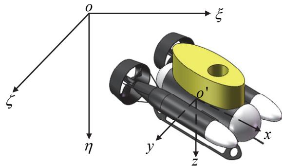
Fig. 1. Coordinate systems for ROV.
