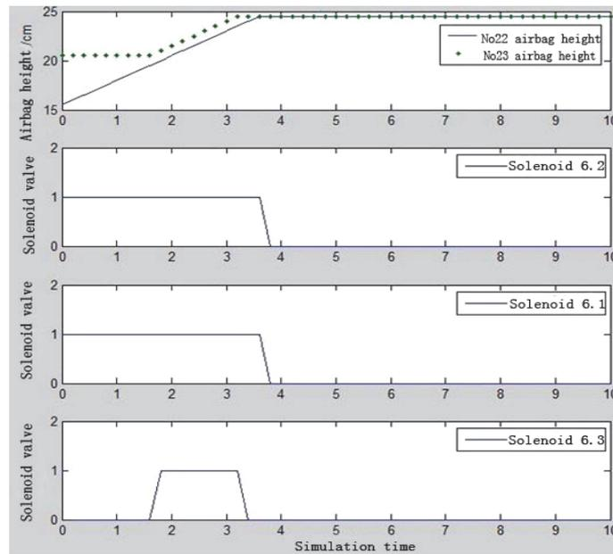
Fig. 4. Simulation Results: when two Airbags'height are lower than target height.
