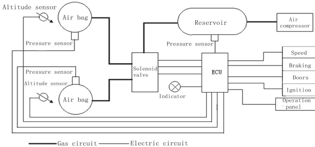
Fig. 1. Structure of the Air Suspension System.
