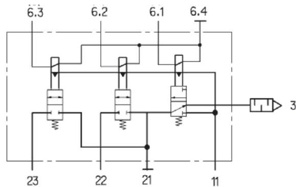
Fig. 2. The Solenoid Valve Circuit of Internal Wiring.
