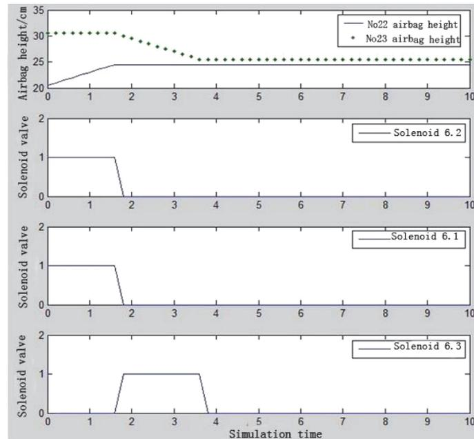
Fig. 5. The Simulation Results: when two Airbags'height are at the both sides of target height.
