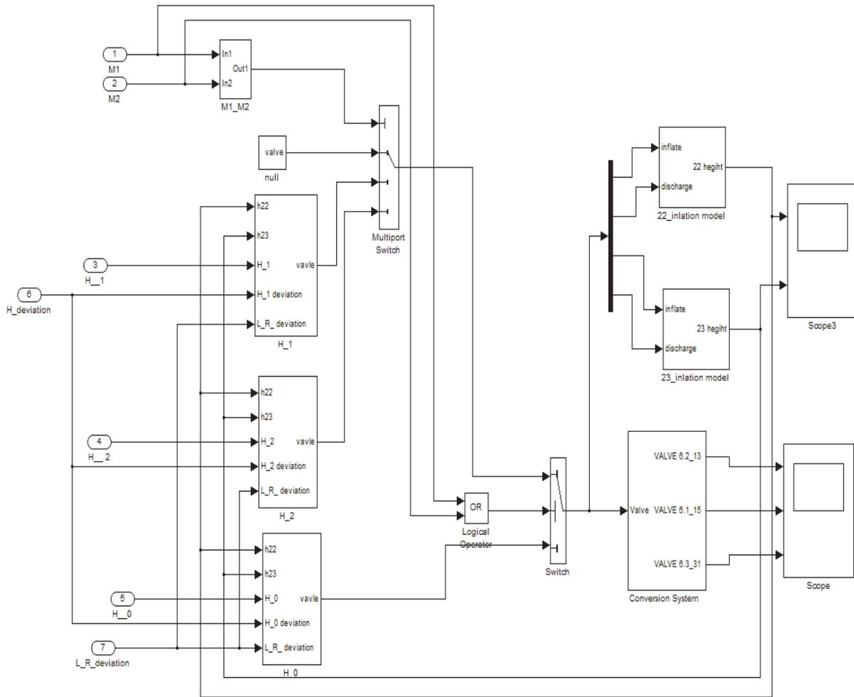
Fig. 3. Simulation Modal in Matlab/Simulink.
