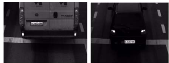
Fig. 2. License plates occur at different heights, but within the range between 30 and 110 centimeters above the ground.
