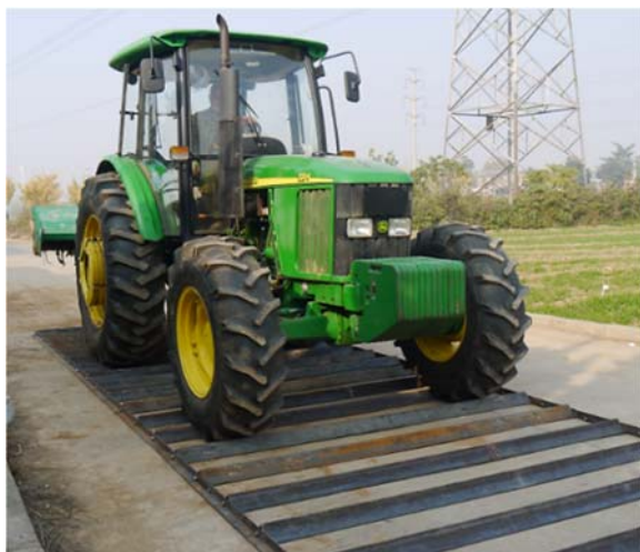
Fig. 5. Tractor four round block test.
