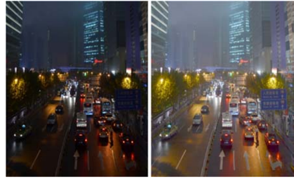
Fig. 6. LIP multiplication. Left: night street image, right: image enhanced by LIP multiplication to maintain an average of 100 (grey level) on the luminance plane.
