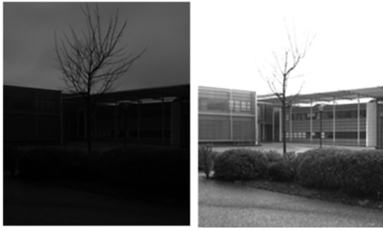
Fig. 4. Simulation of exposure time variation. Left: image acquired at 10 ms, right: simulation of 100 ms exposition applied to the image acquired at 10 ms.
