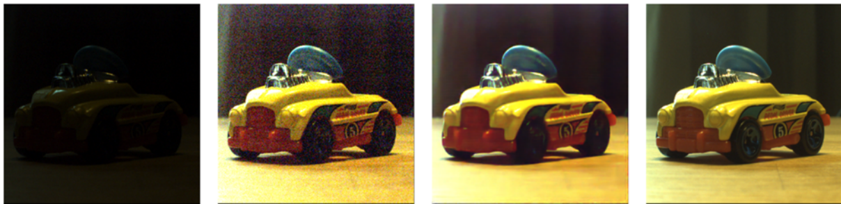
Fig. 11. Application on a color image. From left to right: low exposure acquisition (2 ms), LIP stabilization applied on the low exposure image, noise reduction applied on the enhanced image, high exposure acquisition (clean target, 50 ms).
