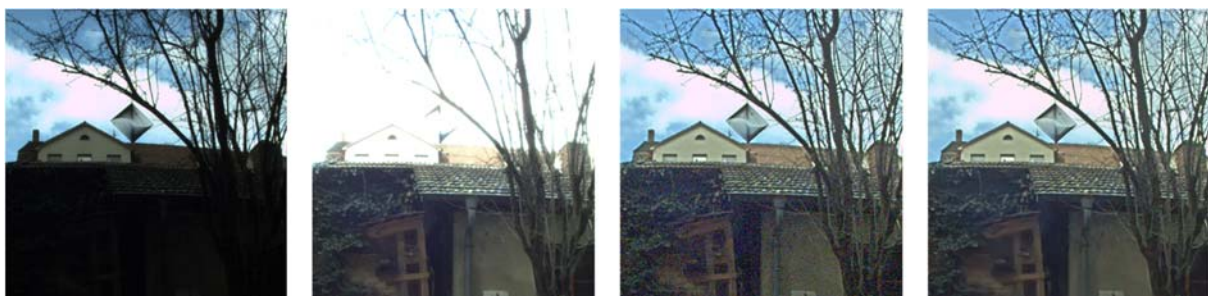
Fig. 12. Brightness spatial stabilization. From left to right, low exposure acquisition (5 ms), higher exposure exposition (50 ms) leading to burned areas, LIP local stabilization applied on the low exposure image, noise reduction applied on the enhanced image.
