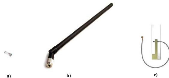
Fig. 7. Three 2.4 GHz off-the-shelf antenna types: a) ceramic integrated SMD (Surface-Mounted Device) antenna, b) SMA (Sub Miniature version A) external dipole antenna, and c) PCB (Printed Circuit Board) antenna.
