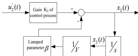
Fig. 5. Humidity control structure block diagram.
