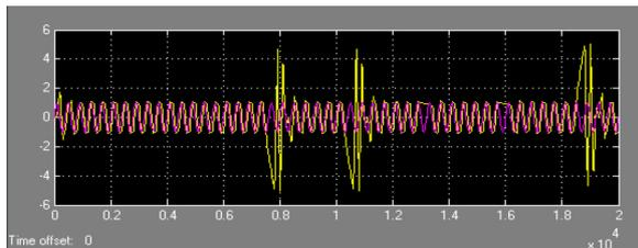
Fig. 8. The control output when the Packet loss rate was 1 % (dotted line is the reference input signal).
