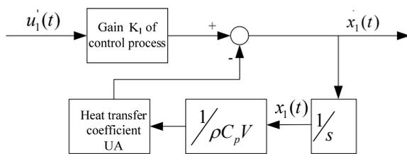
Fig. 4. Temperature control structure block diagram.
