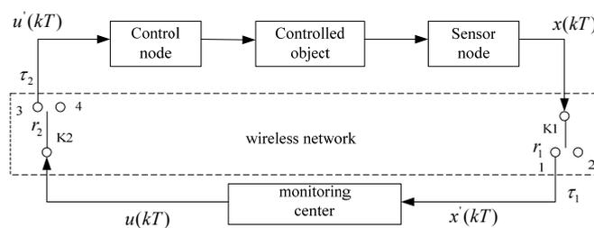
Fig. 3. Model of greenhouse WSN measurement system with time delay and data packet loss.
