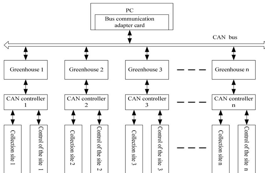
Fig. 1. Greenhouse measurement and control system based on field-bus.
