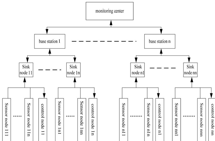
Fig. 2. Greenhouse measurement and control system based on WSN.
