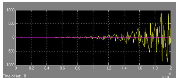
Fig. 12. The control output when the packet loss rate was 35 % (dotted line is the reference input signal).
