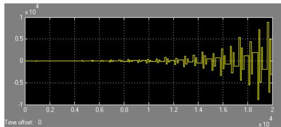
Fig. 11. The control input when the Packet loss rate was 35 %.
