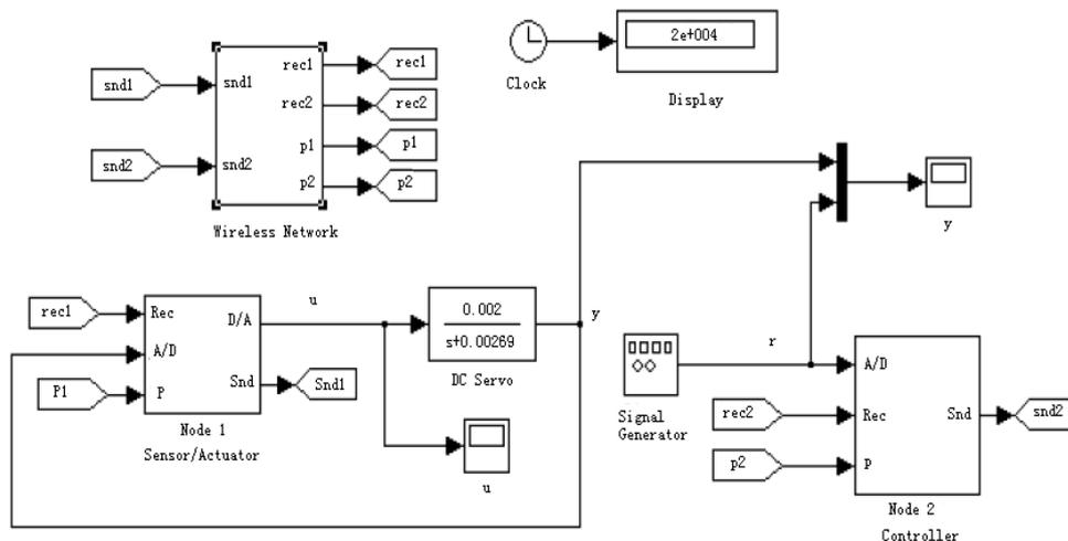
Fig. 6. Greenhouse WSN measurement and control system simulation model.
