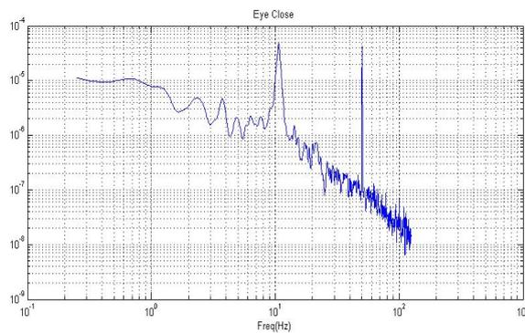
**Fig. 3.** Fourier transform of time domain data showing a broad alpha signal peak at  $\sim 10$  Hz. The participant was asked to close their eyes for period of 40 s. The second peak is the 50 Hz mains signal.
