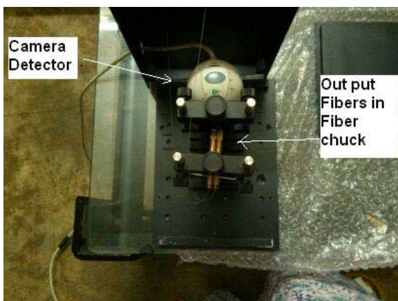
Fig. 5. Detector module mounted on the base plate.
