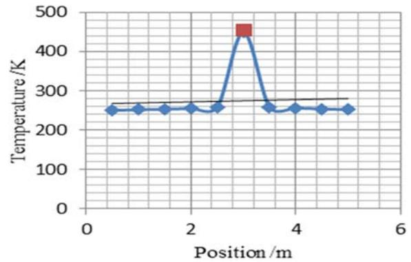
Fig. 7. The result of the temperature measurement from TC 340 (Red colour spike at 3 m position) and the temperature measurement by the proposed method (Blue colour spike at 3 m position).
