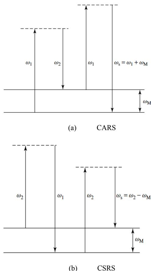
**Fig. 2.** (a) Energy level diagrams for CARS, (b) Energy level diagrams for CSRS.
