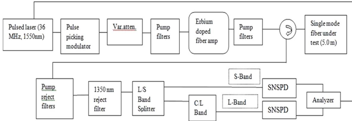
Fig. 3. Measurement set up for wavelength analysis's of coherent anti-Stokes Raman Scattering and coherent stroke Raman Scattering in the fiber under test.
