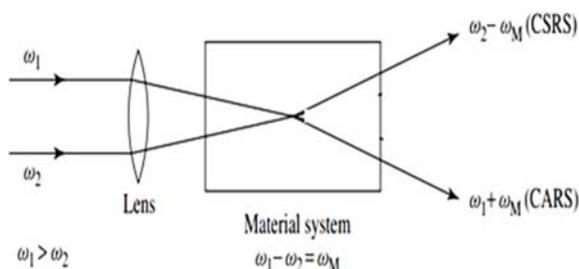
**Fig. 1.** Diagrammatic representations of CARS (coherent anti-Stroke Raman scattering), CSRS (coherent stroke Raman scattering).
