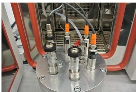
Fig. 3. Cylindrical gas vessel with Trafag density sensors (orange cable connector) and pressure sensor attached in front of a temperature control chamber.
