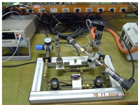
Fig. 4. Manifold with 3 Trafag density sensors (black cable connectors), arranged in a T-configuration, control valves, pressure sensor and vacuum pump (right).
