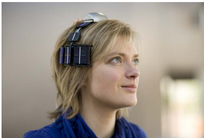
Fig. 11. Wearable wireless EEG system with hybrid power supply.
