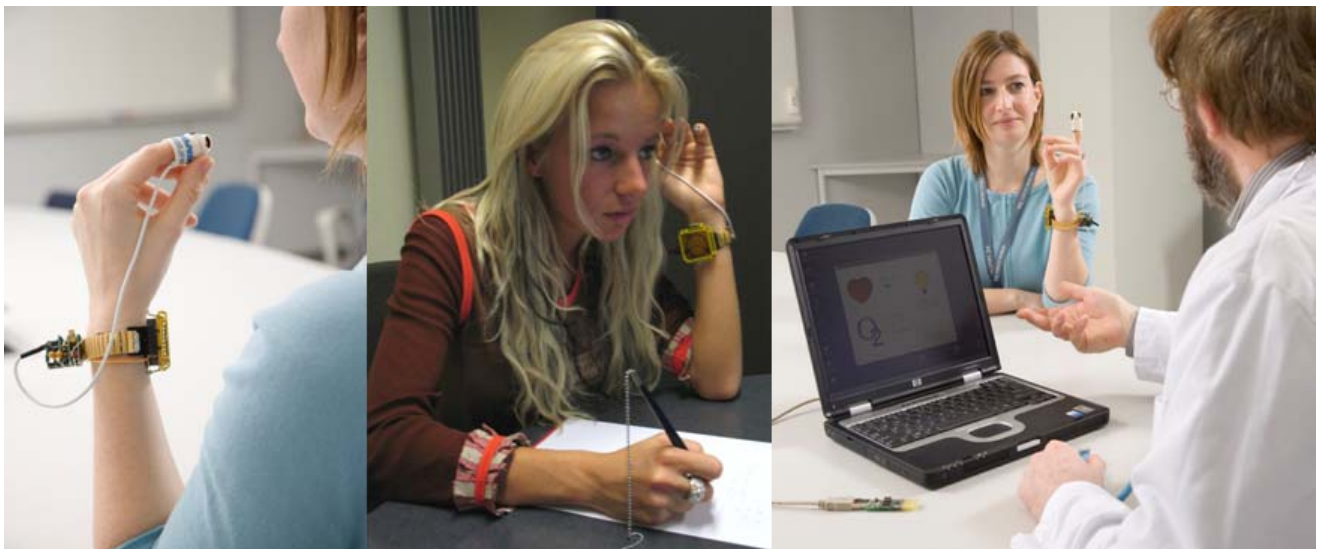
Fig. 3. Body-powered pulse oximeter [4] and the application running on a laptop with a measurement time of 4 s and an update rate of 15 s.
