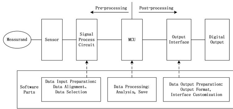
Fig. 1. Basic structure of the gas and coal seam spontaneous combustion sensor experiment device.
