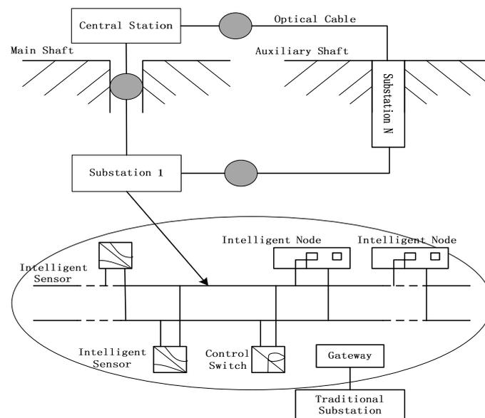
Fig. 2. The mine monitoring system structure based on CAN bus typical.
