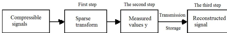
Fig. 1. Compressed sensing theoretical framework.
