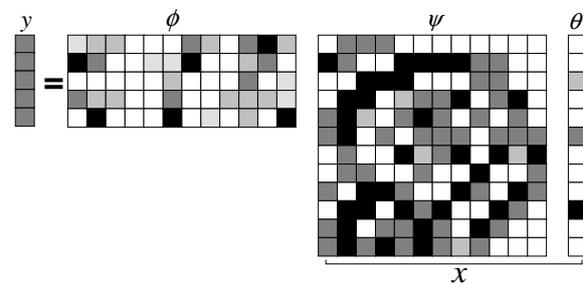
Fig. 2. Compressed sensing linear measurement process.
