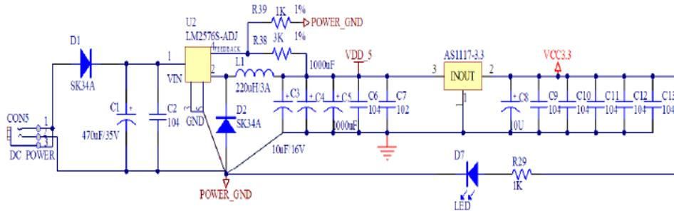
Fig. 5. Schematic diagram of power circuit.
