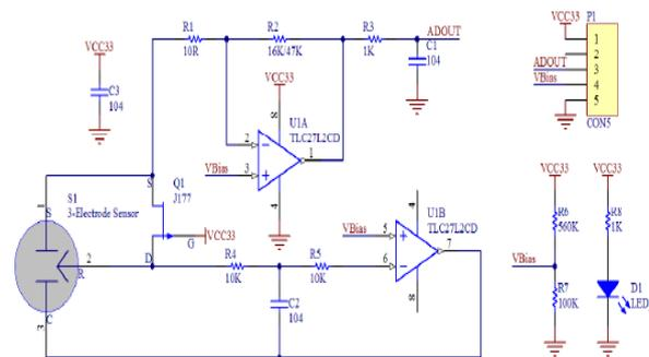
Fig. 4. Measurement circuit of NO<sub>2</sub> and HCHO.
