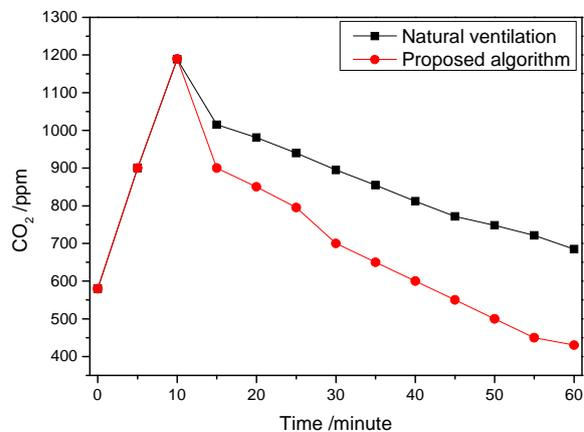
**Fig. 7.** CO<sub>2</sub> monitoring results.
