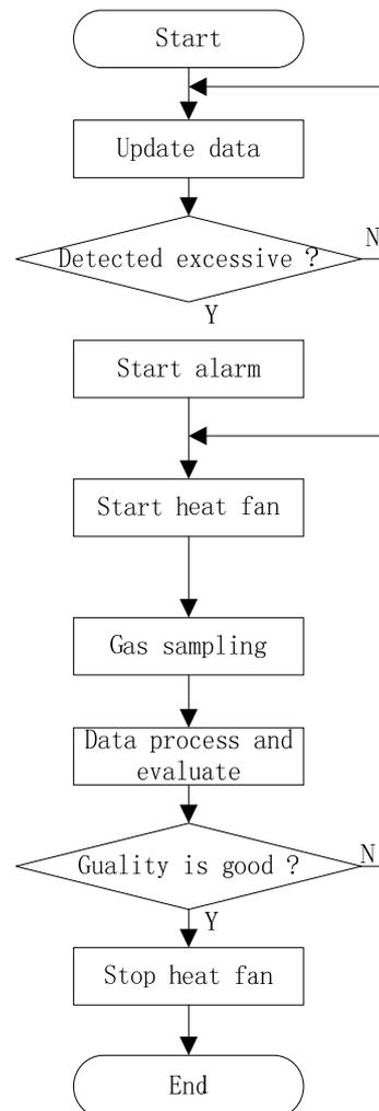
Fig. 6. Flowchart of system working.
