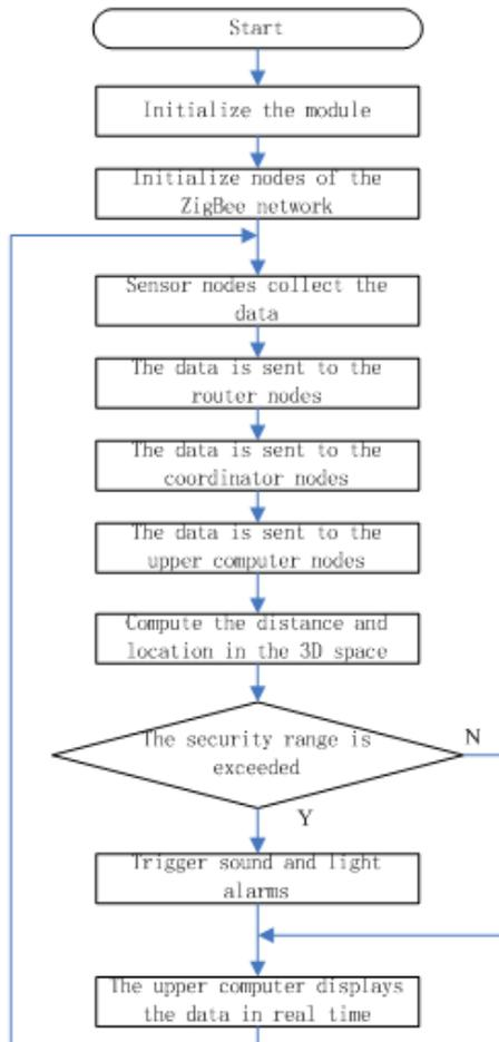
Fig. 7. The system's working flows.
