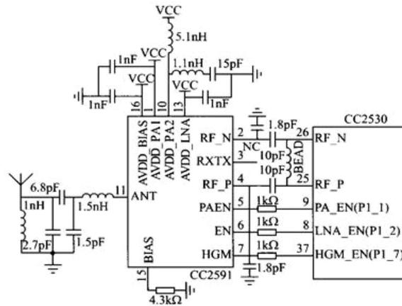
Fig. 2. Hardware interfacing between the CC2530 and CC2591.
