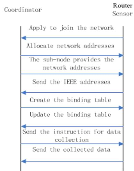
Fig. 8. The creation of the ZigBee network.
