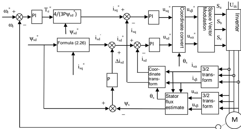
Fig. 2. D-axis control system block diagram based on the current stator flux.
