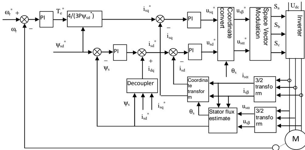
Fig.1. Traditional stator field oriented control system block diagram.
