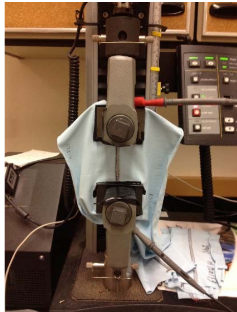
Fig. 8. Experimental setup: sample mounted in Instron with DMM leads attached (top and bottom).
