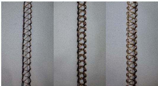
Fig. 7. 2-, 4-, and 5-ply (left to right) bottom-thread coverstitched sensors.
