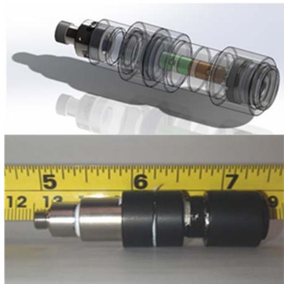
**Fig. 5.** On the top, a model of the passive Q-switch laser and, on the bottom, the finished prototype [26].
