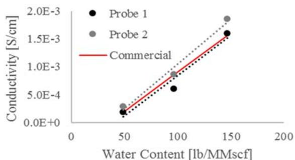
**Fig. 7.** Conductivity of Nafion 117 with water content in 100 psi (0.69 MPa) nitrogen using the homemade (Probs 1 and 2) and commercial probes.
