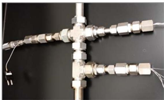
**Fig. 8.** High-pressure flow-through test cell with attached conductivity/corrosion sensors (right side of cell) and thermocouple/pressure transducer (left side of cell).
