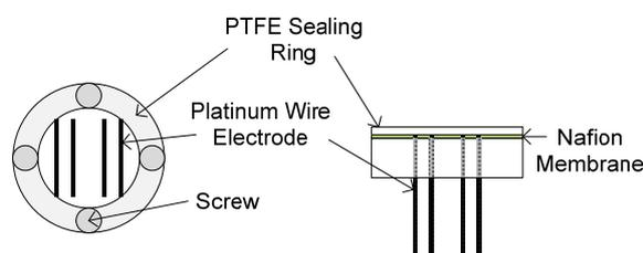
**Fig. 1.** Four-electrode conductivity probe for high-pressure gas systems [3-4].
