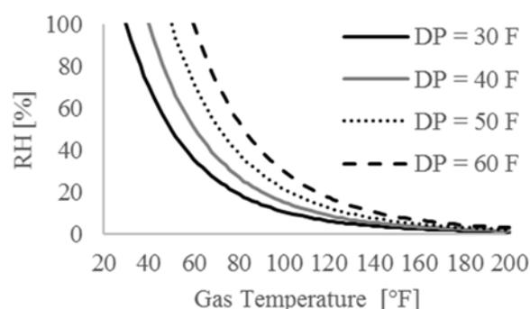
**Fig. 3.** Relative humidity in 1000 psi (6.9 MPa) natural gas as a function of gas and dew point (DP) temperature [5].
