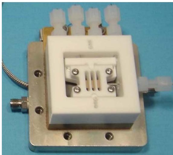
Fig. 5. Low pressure conductivity test cell.
