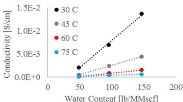
Fig. 6. Conductivity of Nafion 117 with water content in 100 psi (0.69 MPa) nitrogen using the commercial conductivity system [4].
