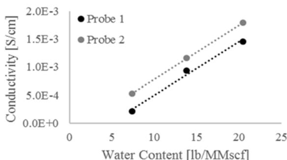
**Fig. 9.** Conductivity of Nafion 117 with water content in 1000 psi (6.9 MPa) nitrogen using the high-pressure conductivity probes [4].
