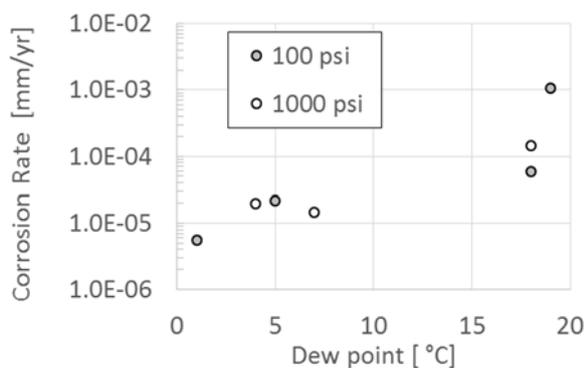
**Fig. 11.** Corrosion rate data for a cell temperature of 60 °C as a function of the dew point for the inlet humidifier.
