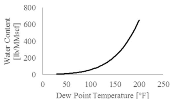
**Fig. 2.** Water content in 1000 psi (6.9 MPa) natural gas as a function of dew point temperature [3].
