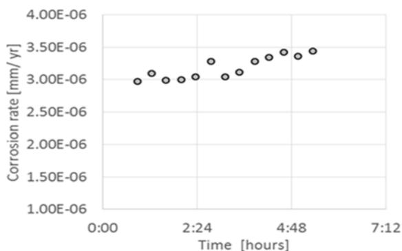
**Fig. 10.** Corrosion rate of a carbon steel wire overtime via LPR on day 3 at 60°C using the modified commercial cell.
